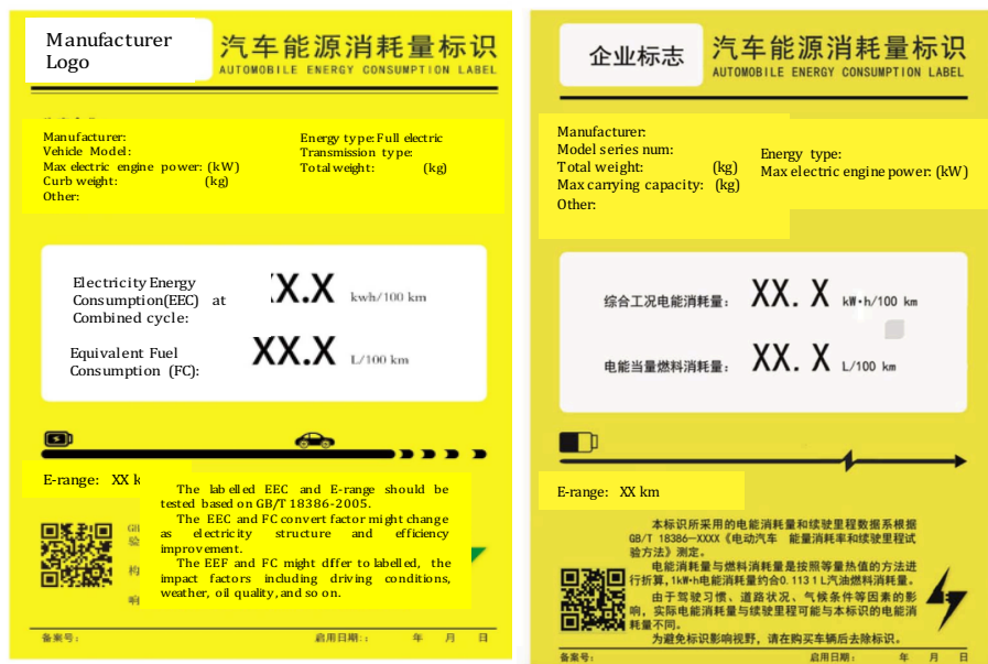
NEV Label: GB 22757.2-DRAFT for PEVs (left), GB 22757.2-2017 for PEVs (right); Main parts were translated to English by iCET
