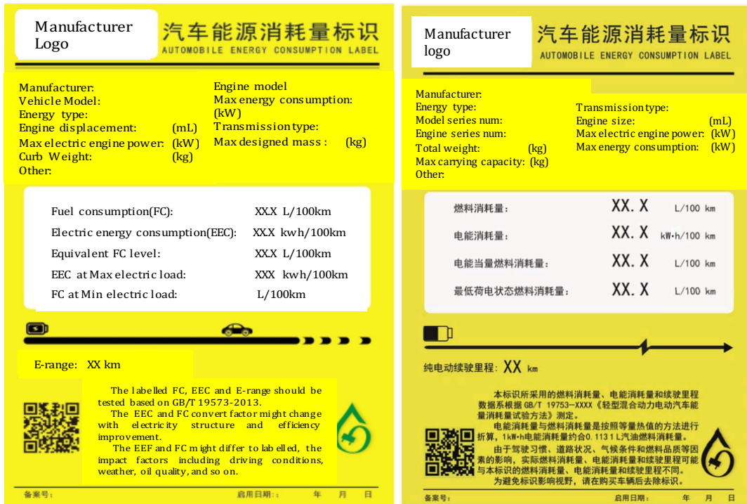
NEV Label: GB 22757.2-DRAFT for PHEVs (left), GB 22757.2-2017 for PHEVs (right); Main parts were translated to English by iCET
